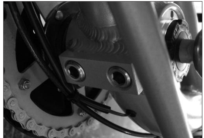
Fig. 7; releasing the cam clamping screws
