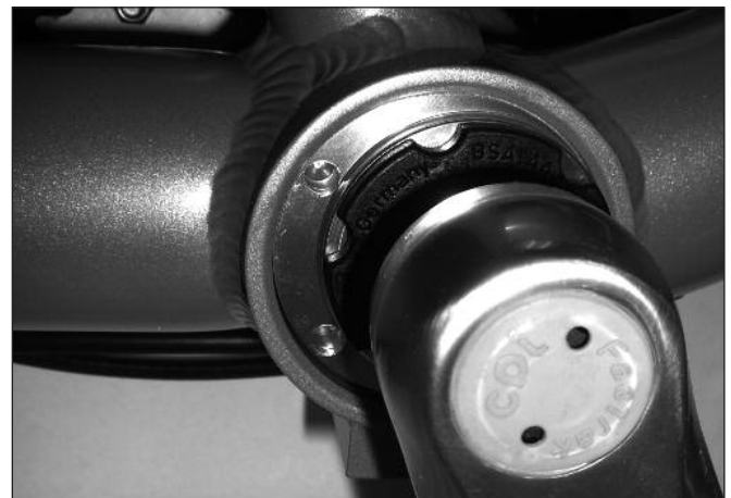
Fig. 7.1; Turning the cam to tension the power transmission chain
